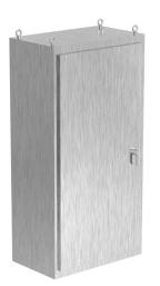
Saginaw NextGen series left enclosure bay, NEMA 3R/4/4X/12/13, 80 x 40 x 24in (HxWxD), freestanding, 316 stainless steel, #4 brush finish, single-door, 3-point padlocking combo handle.
