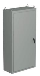
Saginaw NextGen series left enclosure bay, NEMA 3R/4/12/13, 80 x 40 x 18in (HxWxD), freestanding, carbon steel, ANSI 61 gray, polyester powder coat finish, single-door, 3-point padlocking combo handle.
