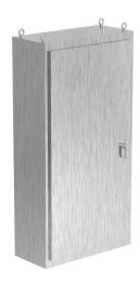
Saginaw NextGen series left enclosure bay, NEMA 3R/4/4X/12/13,  $80 \times 40 \times 18$  in (HxWxD), freestanding, 304 stainless steel, #4 brush finish, single-door, 3-point padlocking combo handle.
