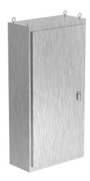
Saginaw NextGen series left enclosure bay, NEMA 3R/4/4X/12/13,  $80 \times 40 \times 18$  in (HxWxD), freestanding, 316 stainless steel, #4 brush finish, single-door, 3-point padlocking combo handle.
