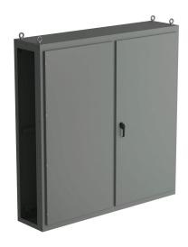
Saginaw NextGen series center enclosure bay, NEMA 3R/12/13,  $80 \times 78 \times 18$  in (HxWxD), freestanding, carbon steel, ANSI 61 gray, polyester powder coat finish, overlapping double-door, 3-point padlocking combo handle.
