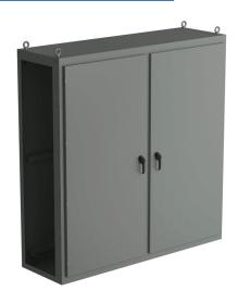
Saginaw NextGen series center enclosure bay, NEMA 3R/4/12/13,  $80 \times 78 \times 24$ in (HxWxD), freestanding, carbon steel, ANSI 61 gray, polyester powder coat finish, 2-door, 3-point padlocking combo handle.
