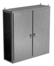
Saginaw NextGen series center enclosure bay, NEMA 3R/4/4X/12/13, 80 x 78 x 24in (HxWxD), freestanding, 304 stainless steel, #4 brush finish, 2-door, 3-point padlocking combo handle.
