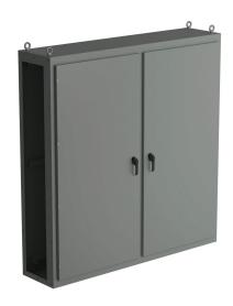
Saginaw NextGen series center enclosure bay, NEMA 3R/4/12/13,  $80 \times 78 \times 18$  in (HxWxD), freestanding, carbon steel, ANSI 61 gray, polyester powder coat finish, 2-door, 3-point padlocking combo handle.
