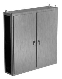
Saginaw NextGen series center enclosure bay, NEMA 3R/4/4X/12/13, 80 x 78 x 18in (HxWxD), freestanding, 304 stainless steel, #4 brush finish, 2-door, 3-point padlocking combo handle.
