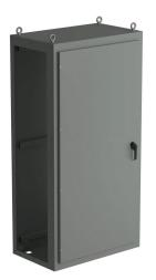
Saginaw NextGen series center enclosure bay, NEMA 3R/4/12/13, 80 x 40 x 24in (HxWxD), freestanding, carbon steel, ANSI 61 gray, polyester powder coat finish, single-door, 3-point padlocking combo handle.
