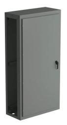
Saginaw NextGen series center enclosure bay, NEMA 3R/4/12/13, 80 x 40 x 18in (HxWxD), freestanding, carbon steel, ANSI 61 gray, polyester powder coat finish, single-door, 3-point padlocking combo handle.
