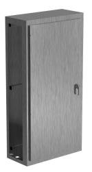
Saginaw NextGen series center enclosure bay, NEMA 3R/4/4X/12/13, 80 x 40 x 18in (HxWxD), freestanding, 304 stainless steel, #4 brush finish, single-door, 3-point padlocking combo handle.
