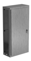
Saginaw NextGen series center enclosure bay, NEMA 3R/4/4X/12/13, 80 x 40 x 18in (HxWxD), freestanding, 316 stainless steel, #4 brush finish, single-door, 3-point padlocking combo handle.
