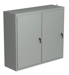
Saginaw NextGen series disconnect enclosure, NEMA 3R/4/12/13, 68 x 78 x 24in (HxWxD), freestanding, carbon steel, ANSI 61 gray, polyester powder coat finish, 2-door, 3-point padlocking combo handle.
