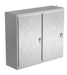
Saginaw NextGen series disconnect enclosure, NEMA 3R/4/4X/12/13, 68 x 78 x 24in (HxWxD), freestanding, 304 stainless steel, #4 brush finish, 2-door, 3-point padlocking combo handle.
