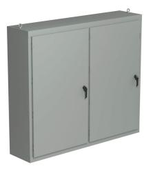
Saginaw NextGen series disconnect enclosure, NEMA 3R/4/12/13, 68 x 78 x 18in (HxWxD), freestanding, carbon steel, ANSI 61 gray, polyester powder coat finish, 2-door, 3-point padlocking combo handle.
