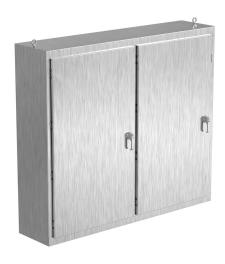
Saginaw NextGen series disconnect enclosure, NEMA 3R/4/4X/12/13, 68 x 78 x 18in (HxWxD), freestanding, 304 stainless steel, #4 brush finish, 2-door, 3-point padlocking combo handle.
