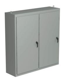
Saginaw NextGen series disconnect enclosure, NEMA 3R/4/12/13, 68 x 66 x 18in (HxWxD), freestanding, carbon steel, ANSI 61 gray, polyester powder coat finish, 2-door, 3-point padlocking combo handle.
