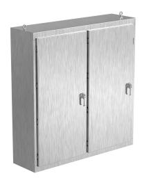
Saginaw NextGen series disconnect enclosure, NEMA 3R/4/4X/12/13, 68 x 66 x 18in (HxWxD), freestanding, 304 stainless steel, #4 brush finish, 2-door, 3-point padlocking combo handle.
