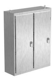
Saginaw NextGen series disconnect enclosure, NEMA 3R/4/4X/12/13, 68 x 54 x 18in (HxWxD), freestanding, 304 stainless steel, #4 brush finish, 2-door, 3-point padlocking combo handle.
