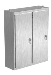
Saginaw NextGen series disconnect enclosure, NEMA 3R/4/4X/12/13, 68 x 54 x 18in (HxWxD), freestanding, 316 stainless steel, #4 brush finish, 2-door, 3-point padlocking combo handle.
