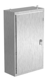
Saginaw NextGen series disconnect enclosure, NEMA 3R/4/4X/12/13, 68 x 40 x 18in (HxWxD), freestanding, 304 stainless steel, #4 brush finish, single-door, 3-point padlocking combo handle.
