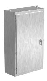
Saginaw NextGen series disconnect enclosure, NEMA 3R/4/4X/12/13, 68 x 40 x 18in (HxWxD), freestanding, 316 stainless steel, #4 brush finish, single-door, 3-point padlocking combo handle.
