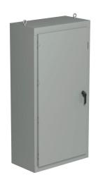
Saginaw NextGen series disconnect enclosure, NEMA 3R/4/12/13, 68 x 34 x 18in (HxWxD), freestanding, carbon steel, ANSI 61 gray, polyester powder coat finish, single-door, 3-point padlocking combo handle.
