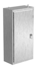
Saginaw NextGen series disconnect enclosure, NEMA 3R/4/4X/12/13, 68 x 34 x 18in (HxWxD), freestanding, 316 stainless steel, #4 brush finish, single-door, 3-point padlocking combo handle.
