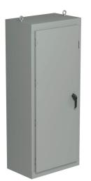
Saginaw NextGen series disconnect enclosure, NEMA 3R/4/12/13, 68 x 28 x 18in (HxWxD), freestanding, carbon steel, ANSI 61 gray, polyester powder coat finish, single-door, 3-point padlocking combo handle.
