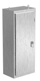
Saginaw NextGen series disconnect enclosure, NEMA 3R/4/4X/12/13, 68 x 28 x 18in (HxWxD), freestanding, 304 stainless steel, #4 brush finish, single-door, 3-point padlocking combo handle.
