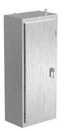
Saginaw NextGen series disconnect enclosure, NEMA 3R/4/4X/12/13, 68 x 28 x 18in (HxWxD), freestanding, 316 stainless steel, #4 brush finish, single-door, 3-point padlocking combo handle.
