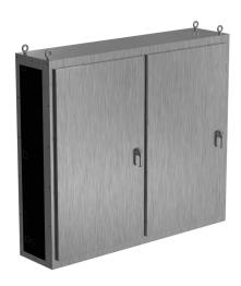
Saginaw NextGen series right disconnect enclosure bay, NEMA 3R/4/4X/12/13, 68 x 78 x 18in (HxWxD), freestanding, 304 stainless steel, #4 brush finish, 2-door, 3-point padlocking combo handle.
