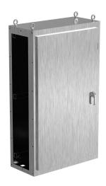
Saginaw NextGen series right disconnect enclosure bay, NEMA 3R/4/4X/12/13, 68 x 40 x 18in (HxWxD), freestanding, 304 stainless steel, #4 brush finish, single-door, 3-point padlocking combo handle.
