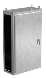
Saginaw NextGen series right disconnect enclosure bay, NEMA 3R/4/4X/12/13, 68 x 40 x 18in (HxWxD), freestanding, 316 stainless steel, #4 brush finish, single-door, 3-point padlocking combo handle.
