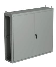
Saginaw NextGen series right enclosure bay, NEMA 3R/12/13, 68 x 78 x 18in (HxWxD), freestanding, carbon steel, ANSI 61 gray, polyester powder coat finish, overlapping double-door, 3-point padlocking combo handle.
