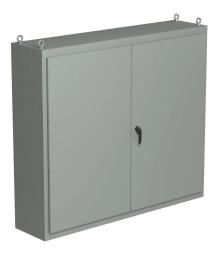
Saginaw NextGen series left enclosure bay, NEMA 3R/12/13, 68 x 78 x 18in (HxWxD), freestanding, carbon steel, ANSI 61 gray, polyester powder coat finish, overlapping double-door, 3-point padlocking combo handle.
