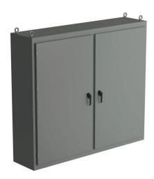
Saginaw NextGen series left enclosure bay, NEMA 3R/4/12/13, 68 x 78 x 18in (HxWxD), freestanding, carbon steel, ANSI 61 gray, polyester powder coat finish, 2-door, 3-point padlocking combo handle.
