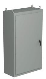
Saginaw NextGen series left enclosure bay, NEMA 3R/4/12/13, 68 x 40 x 18in (HxWxD), freestanding, carbon steel, ANSI 61 gray, polyester powder coat finish, single-door, 3-point padlocking combo handle.
