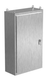
Saginaw NextGen series left enclosure bay, NEMA 3R/4/4X/12/13,  $68 \times 40 \times 18$  in (HxWxD), freestanding, 304 stainless steel, #4 brush finish, single-door, 3-point padlocking combo handle.
