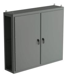
Saginaw NextGen series center enclosure bay, NEMA 3R/4/12/13, 68 x 78 x 18in (HxWxD), freestanding, carbon steel, ANSI 61 gray, polyester powder coat finish, 2-door, 3-point padlocking combo handle.
