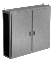
Saginaw NextGen series center enclosure bay, NEMA 3R/4/4X/12/13, 68 x 78 x 18in (HxWxD), freestanding, 304 stainless steel, #4 brush finish, 2-door, 3-point padlocking combo handle.
