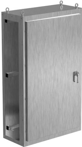
Saginaw NextGen series center enclosure bay, NEMA 3R/4/4X/12/13, 68 x 40 x 18in (HxWxD), freestanding, 304 stainless steel, #4 brush finish, single-door, 3-point padlocking combo handle.
