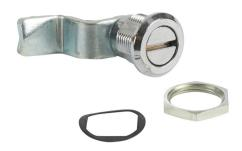
Saginaw enclosure latch, replacement, slotted, miniature 1/4-turn, 1-point, die-cast zinc, chrome finish. For use with Enviroline Junction series enclosures and deep-hinged doors. (1) SCE-105419 cam included.
