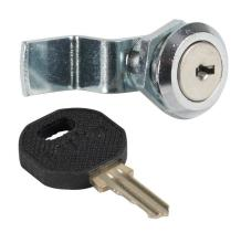
Saginaw enclosure latch, replacement, keylocking, miniature 1/4-turn, 1-point, die-cast zinc, chrome finish. For use with Enviroline Junction series enclosures and deep-hinged doors. (1) SCE-2233X key included.
