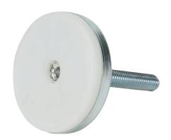
Saginaw leveling pad, zinc-plated steel with a plastic base. Package of 4. 3/8 - 16 threads, 2 in height.
