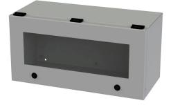
Saginaw wiring trough,  $8 \times 9 \times 18$  in (HxDxL), NEMA 3R/4/12/13, wall mount, carbon steel, ANSI 61 gray, powder coat finish, single-door, polycarbonate window.
