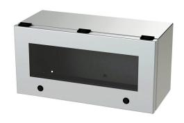
Saginaw wiring trough, 8 x 9 x 18in (HxDxL), NEMA 3R/4/4X/12/13, wall mount, 304 stainless steel, #4 brush finish, single-door, polycarbonate window.
