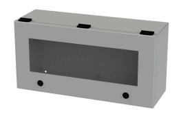
Saginaw wiring trough, 6 x 9 x 18in (HxDxL), NEMA 3R/4/12/13, wall mount, carbon steel, ANSI 61 gray, powder coat finish, single-door, polycarbonate window.
