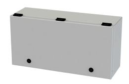
Saginaw wiring trough,  $6 \times 9 \times 18$ in (HxDxL), NEMA 3R/4/12/13, wall mount, carbon steel, RAL 7035 light gray, powder coat finish, single-door.
