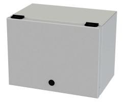
Saginaw wiring trough, 8 x 9 x 12in (HxDxL), NEMA 3R/4/12/13, wall mount, carbon steel, RAL 7035 light gray, powder coat finish, single-door.
