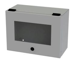
Saginaw wiring trough,  $6 \times 9 \times 12$ in (HxDxL), NEMA 3R/4/12/13, wall mount, carbon steel, ANSI 61 gray, powder coat finish, single-door, polycarbonate window.
