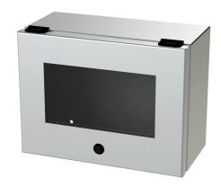
Saginaw wiring trough, 6 x 9 x 12in (HxDxL), NEMA 3R/4/4X/12/13, wall mount, 304 stainless steel, #4 brush finish, single-door, polycarbonate window.
