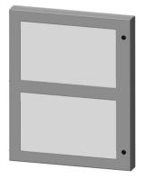
Saginaw universal deep-hinged door, NEMA 3R/12/13, 28.00 x 22.00 x 2.63in, carbon steel, ANSI 61 gray, concealed hinges, polycarbonate window. For use with wall-mount enclosures.
